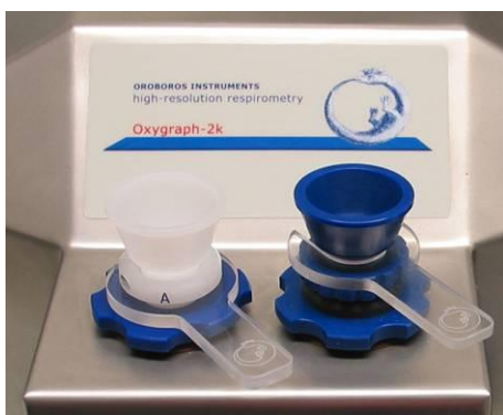
Figure 1. Stopper-spacers used for air calibration with the PVDF stopper (Chamber A) or titanium stopper (Chamber B).
