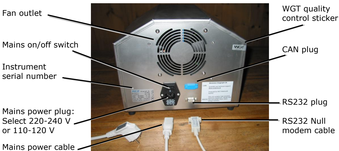
Series A: Rear of the Oxygraph-2k main unit
