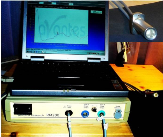
Figure 1: Whitland Research RM200 lightguide spectrophotometer and the LEA stopper (enlarged top right).
