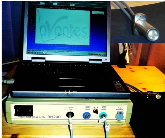
Figure 1: Whitland Research RM200 lightguide spectrophotometer and the LEA stopper (enlarged top right).
