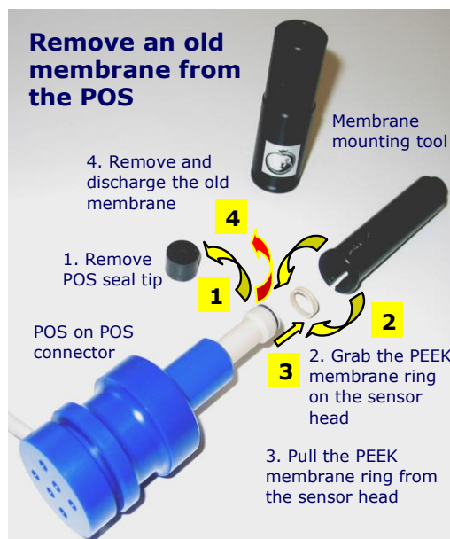
Figure 2. Removal of a used membrane from the POS.
