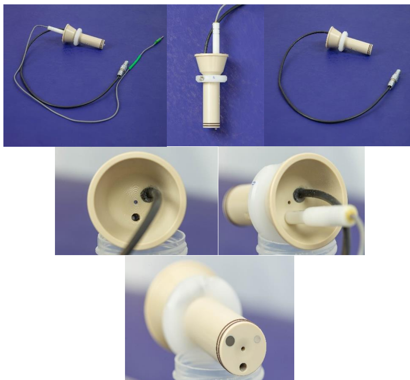
Figure 2. Q-Sensor assembly. First row from left to the right: Q-Sensor with the reference electrode, Q-Stopper without the reference electrode. Second row: Q-Stopper viewed from above without and with the reference electrode. Third row: Q-Stopper viewed from bottom. Glassy carbon electrode (black) and platinum electrode (shiny, silver) are built-in part of the stopper. One gas-escape/titration capillary and an inlet for the reference electrode can be seen.
