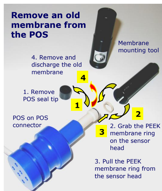
Figure 2. Removal of a used membrane from the POS.
